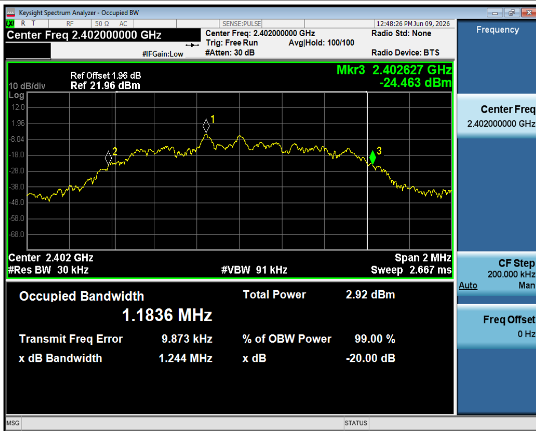
-20dB Bandwidth NVNT 2-DH1 2402MHz Ant1
