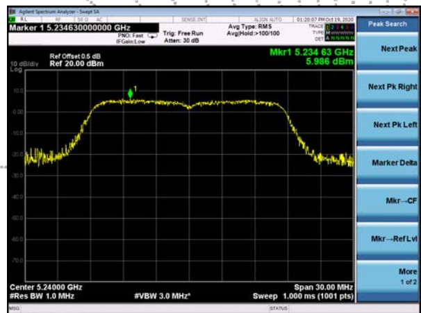
(802.11ac20) PSD plot on channel 48
