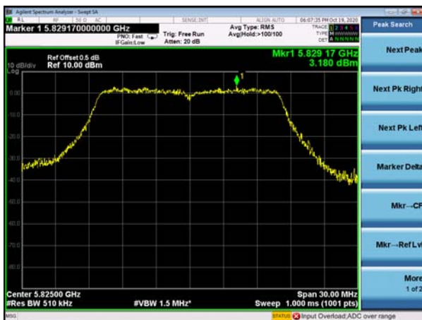
(802.11a) PSD plot on channel 165
