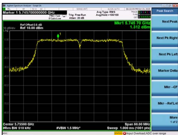
(802.11ac40) PSD plot on channel 159
