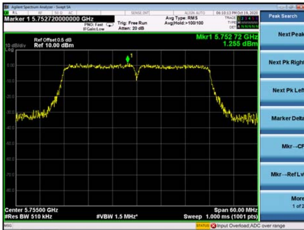
(802.11n40) PSD plot on channel 159
