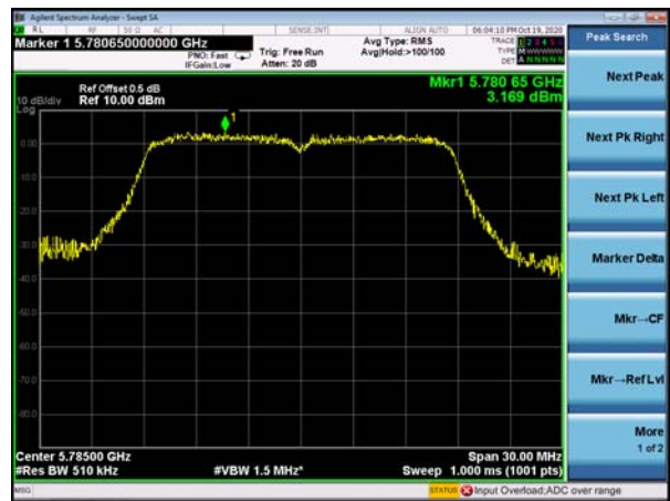
(802.11n20) PSD plot on channel 165
