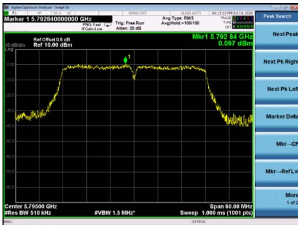
(802.11n40) PSD plot on channel 159
