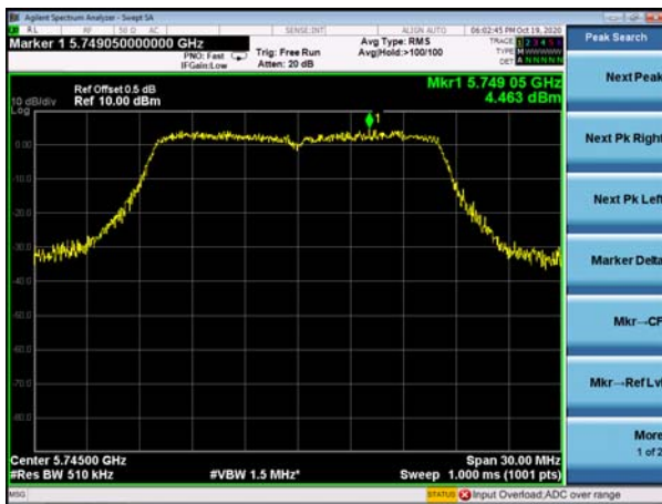
(802.11a) PSD plot on channel 157
