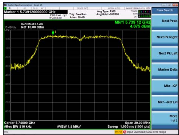
(802.11n20) PSD plot on channel 157
