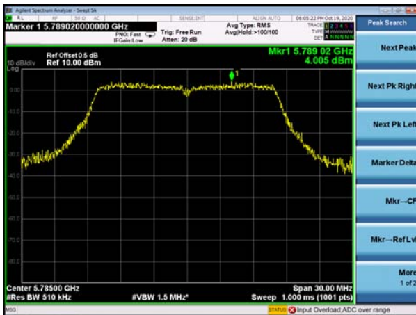
(802.11a) PSD plot on channel 165
