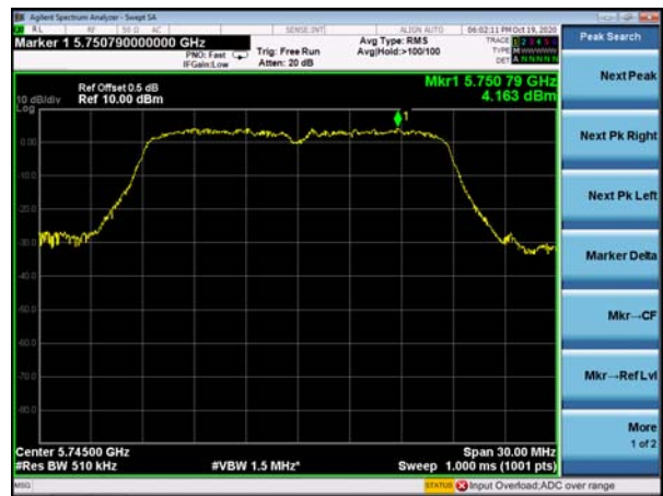
(802.11ac20) PSD plot on channel 157
