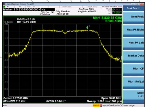
(802.11ac20) PSD plot on channel 165
