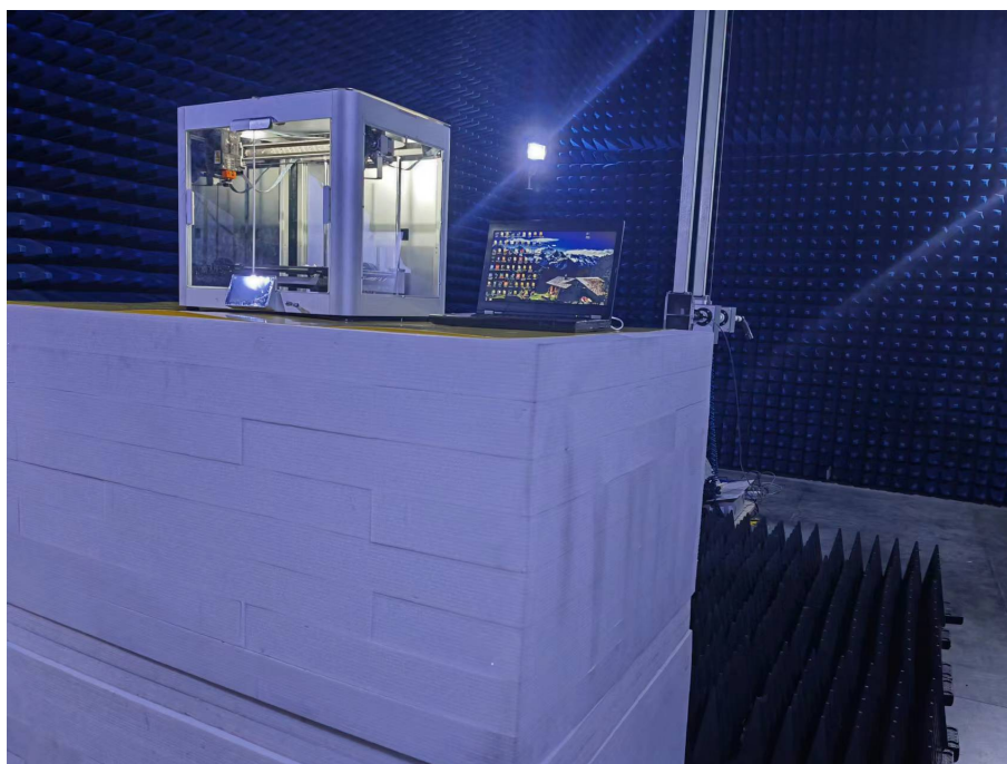
Photo of Radiated Emission Measurement (Above 1G)
