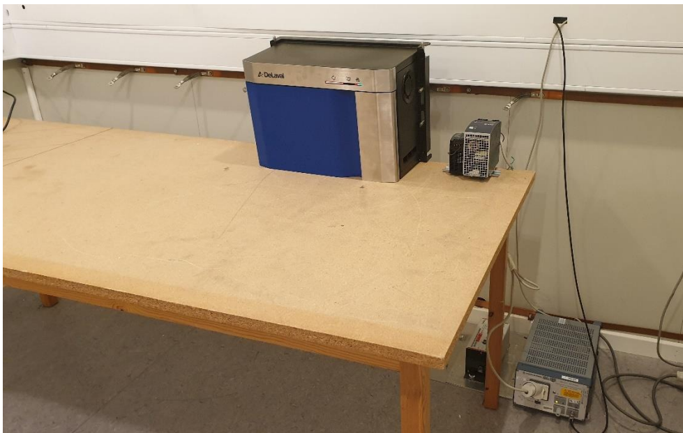
Photo 9. AC Conducted emission test set up.
