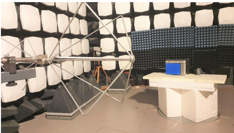
Photo 7. Radiated emission test setup in SAC. 30 - 200 MHz.
