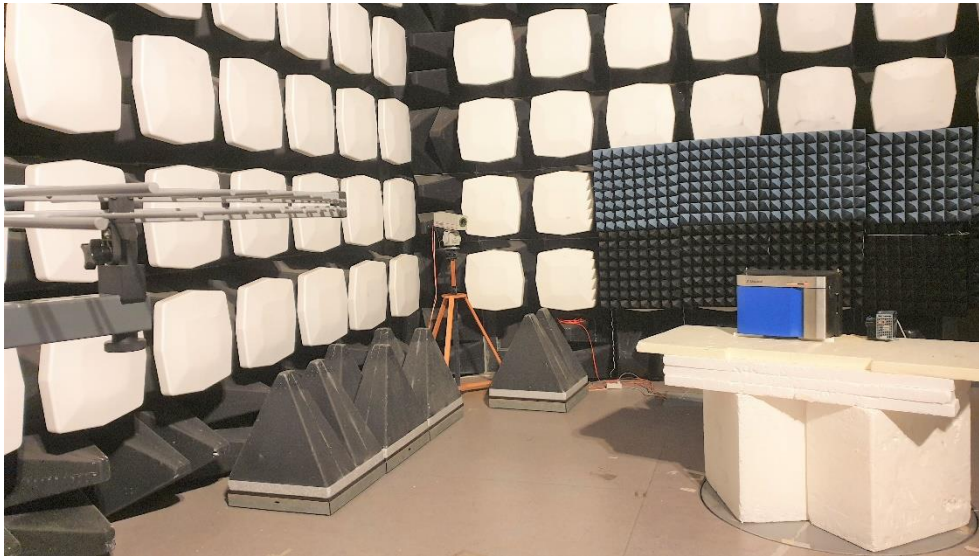
Photo 8. Radiated emission test setup in SAC. 200 - 1000 MHz.
