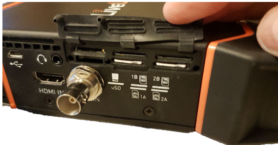
SIMs Installed in the LU300S “A” Slots
