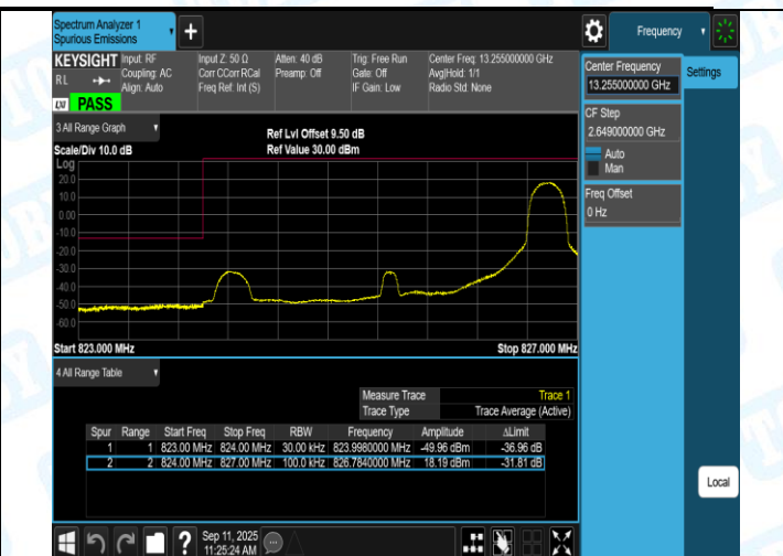
Band5-3MHz-16QAM-20635-1RB#0-PASS
