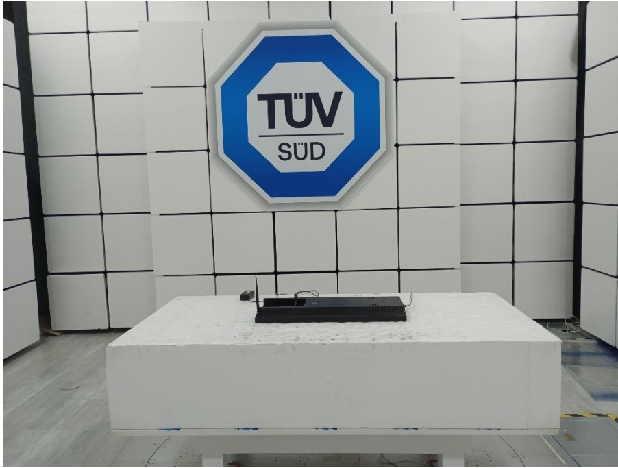
Set-up for Spurious Emissions Front View
