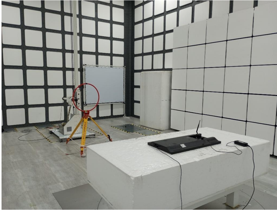
Set-up for Spurious Emissions Rear View
