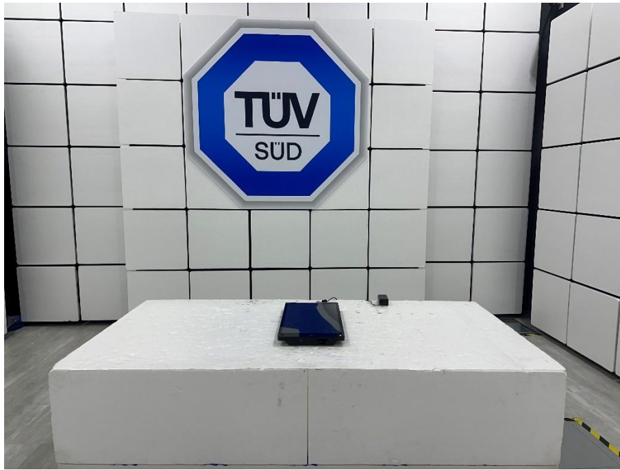
Set-up for Spurious Emissions Front View
