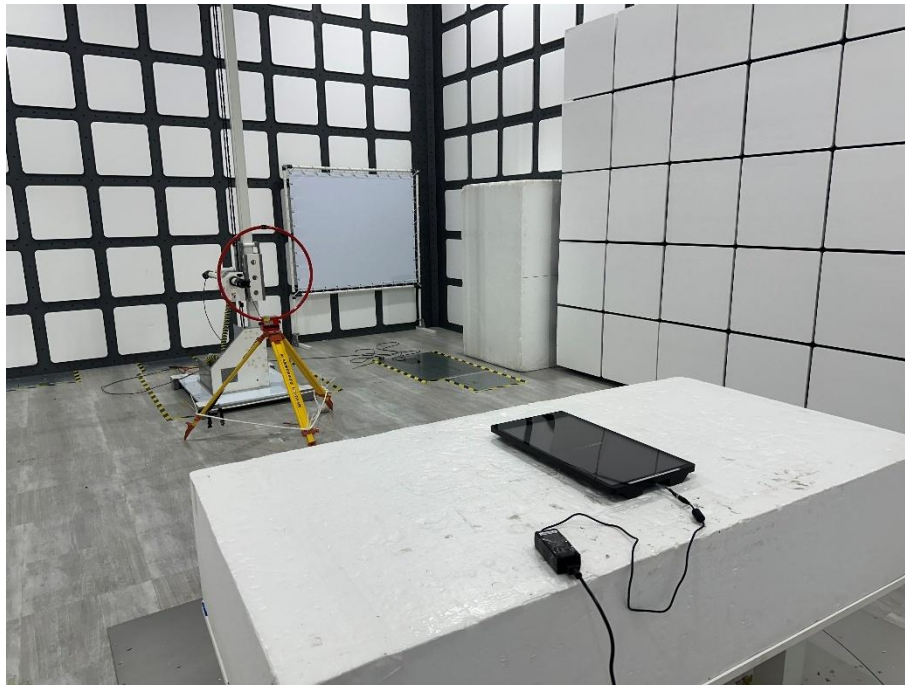
Set-up for Spurious Emissions Rear View
