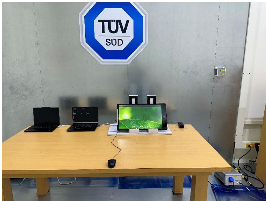
Set-up for Conduction Emission Front View
