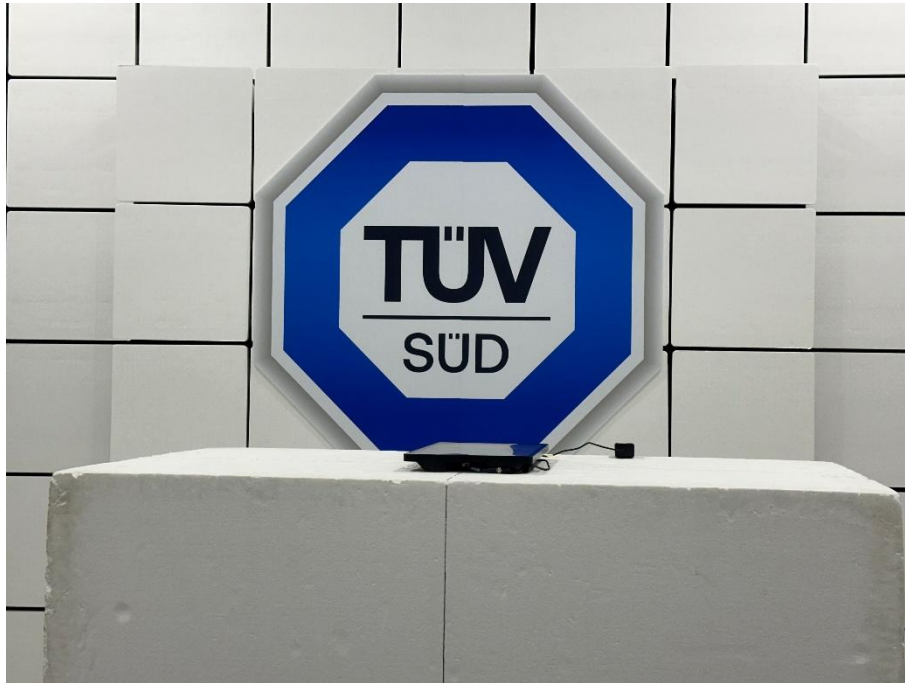
Set-up for Spurious Emissions Front View
