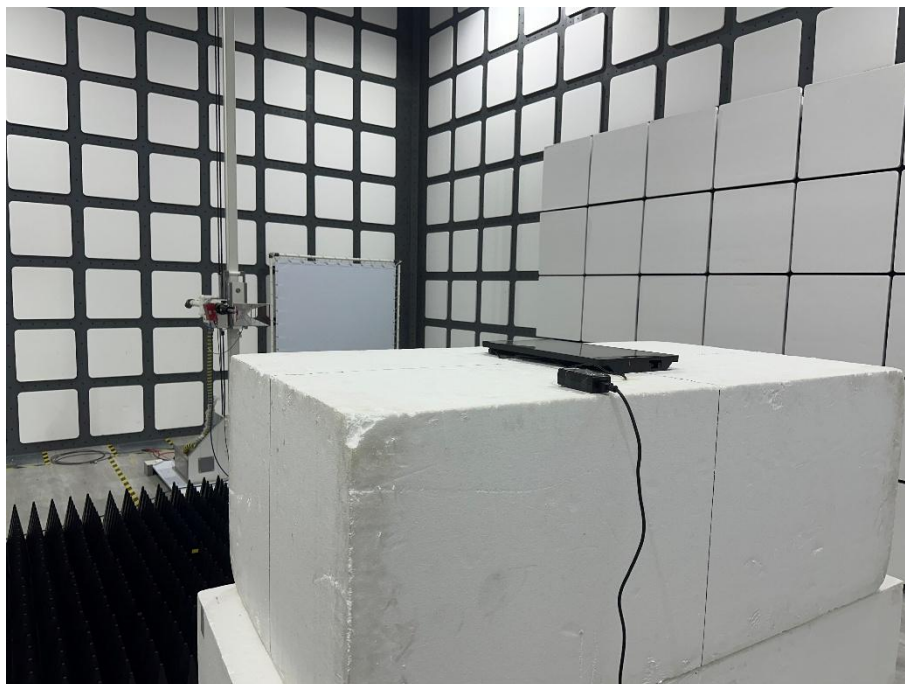
Set-up for Spurious Emissions Rear View
