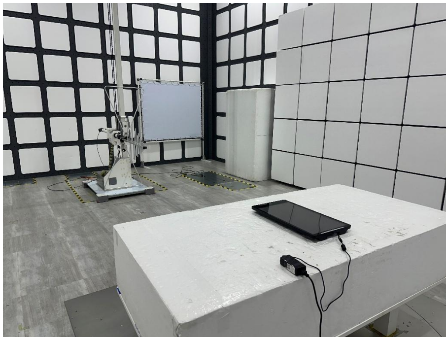
Set-up for Spurious Emissions Rear View
