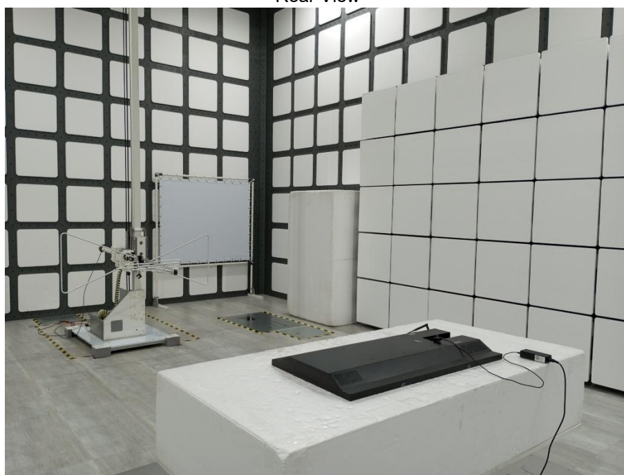
Set-up for Spurious Emissions Rear View
