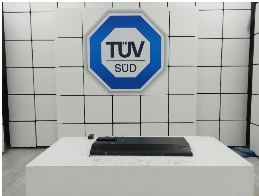
Set-up for Spurious Emissions Front View
