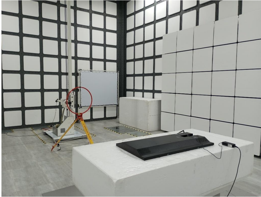
Set-up for Spurious Emissions Rear View
