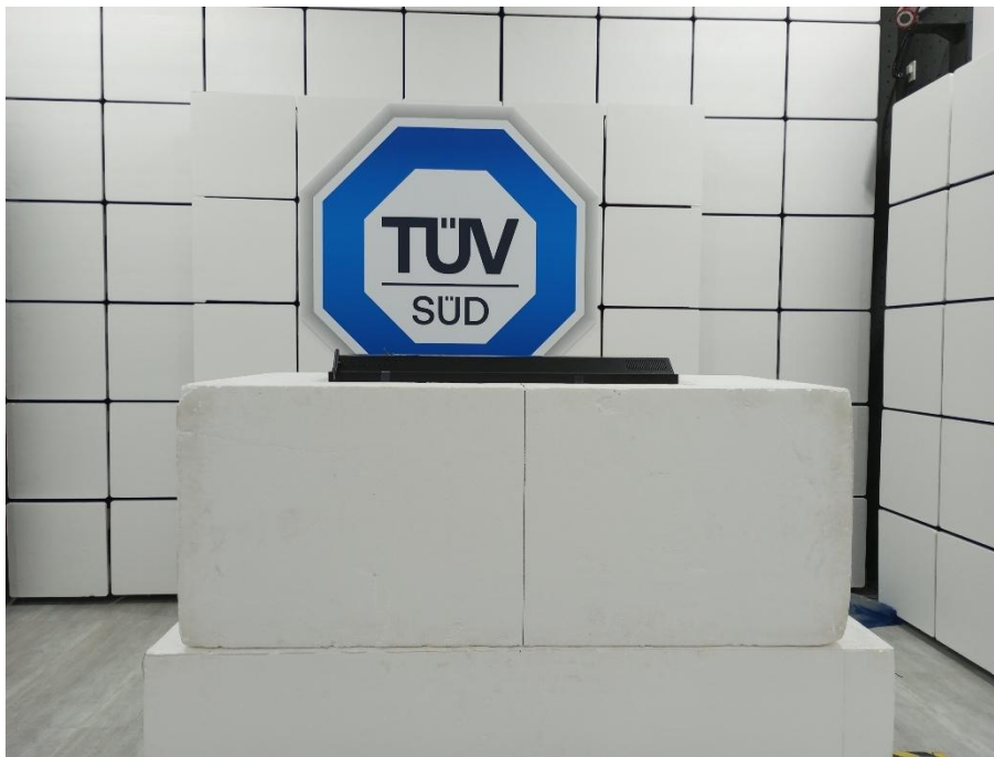
Set-up for Spurious Emissions Front View
