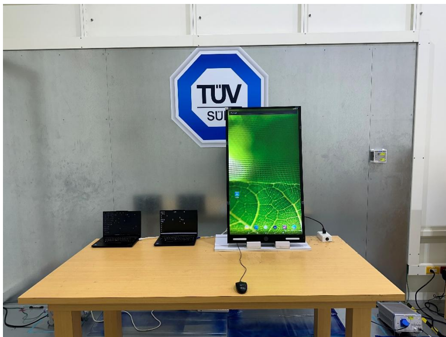
Set-up for Conduction Emission Front View
