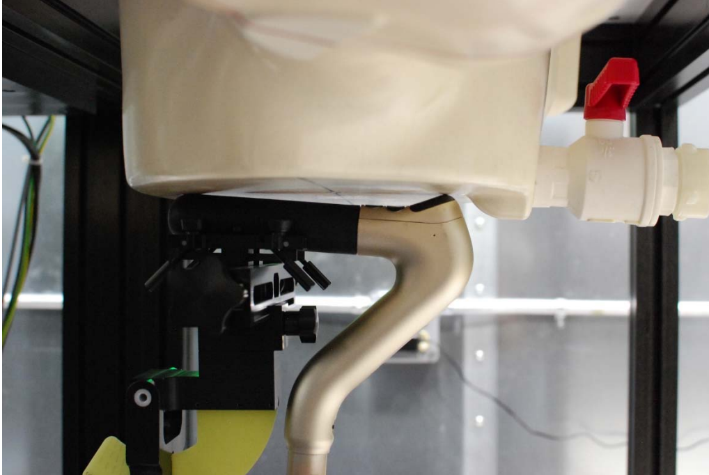
SAR Test Setup Photo 2 – Body, Top Side at 0mm
