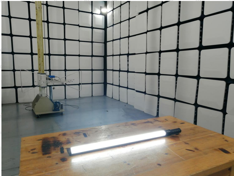
Photo of Radiation Emission Test
