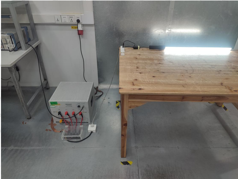
Photo of Conducted Emission Measurement
