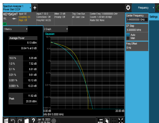
Ant 0_20M_QPSK_FULLRB_PAPR_Middle channel
