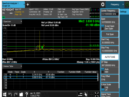
Ant 2_20M_QPSK_1RB0_CSE2_High channel
