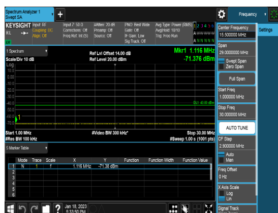
Ant 2_20M_QPSK_FULLRB_CSE0b_Low channel
