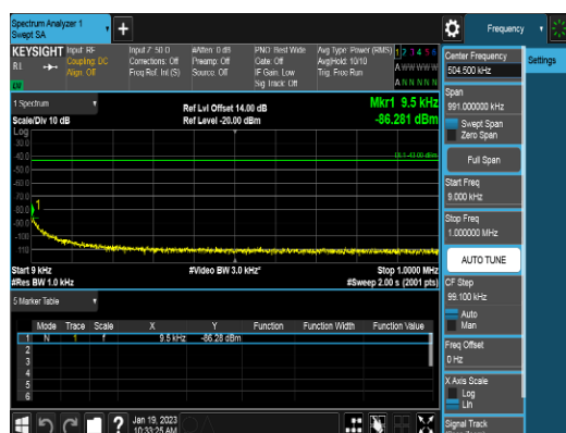
Ant 2_20M_QPSK_FULLRB_CSE0b_Low channel
