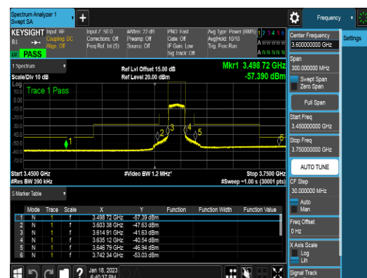
Ant 2_20M_QPSK_FULLLRB_CSEpart96_Middle channel
