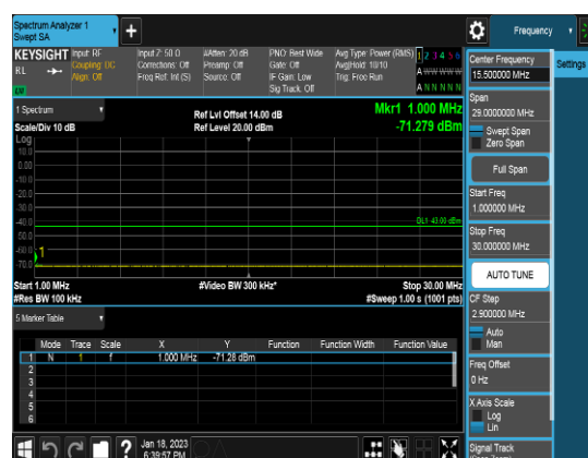
Ant 2_20M_QPSK_FULLRB_CSE0b_Middle channel
