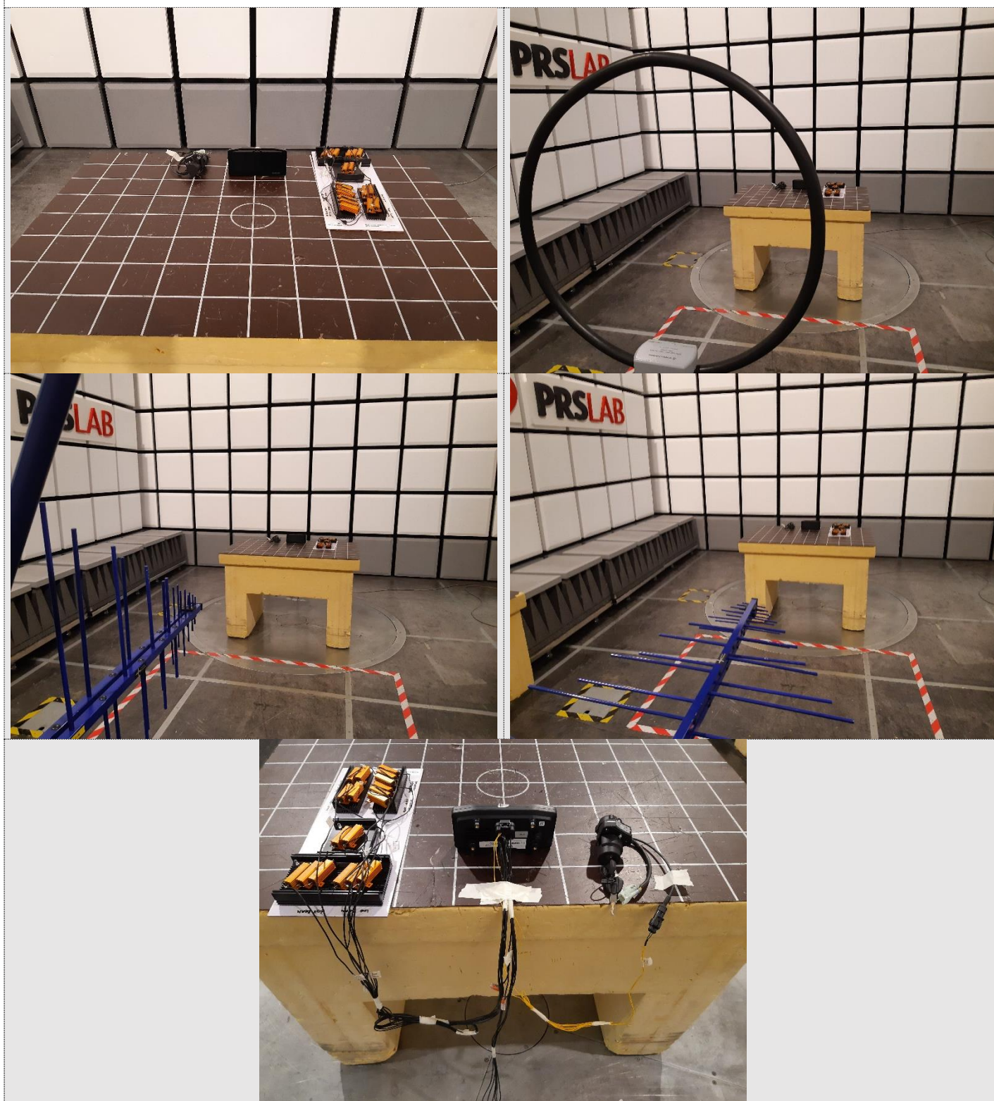
PHOTO N° 2 - RADIATED EMISSION TEST SETUP
