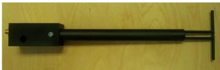
Figure 1 – MVG COMOSAR Validation Dipole
