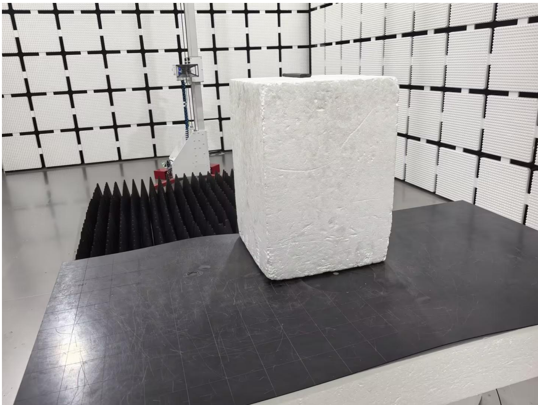
Spurious Emission above 1GHz test photo
