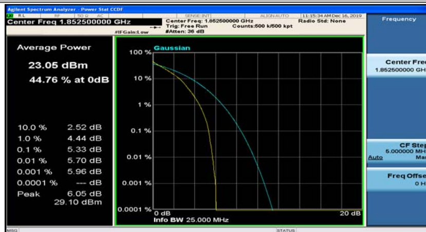
(Channel Bandwidth: 5 MHz)_LCH_QPSK_25RB#0
