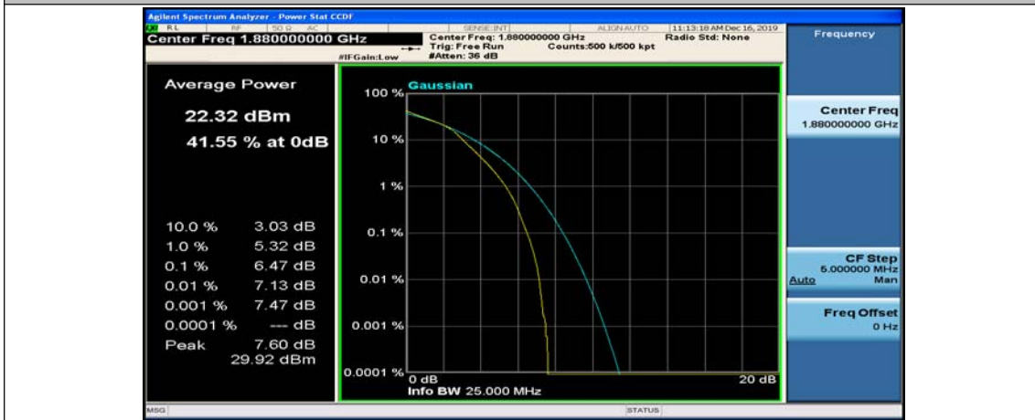
(Channel Bandwidth: 3 MHz)_MCH_16QAM_15RB#0
