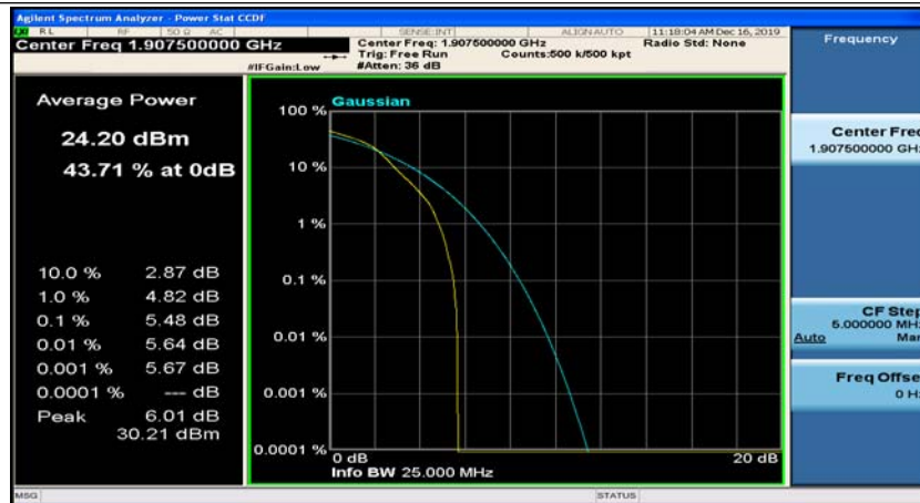
(Channel Bandwidth: 5 MHz)_HCH_16QAM_1RB#24
