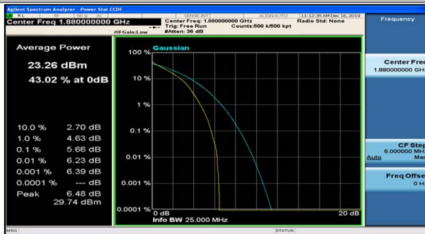
(Channel Bandwidth: 3 MHz)_MCH_QPSK_8RB#4
