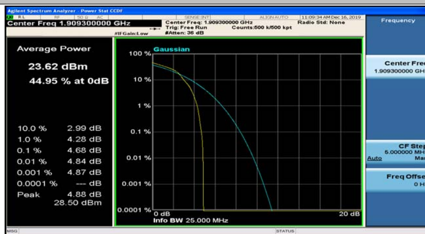
(Channel Bandwidth: 1.4 MHz)_HCH_16QAM_3RB#0
