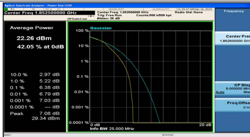
(Channel Bandwidth: 5 MHz)_LCH_16QAM_12RB#13
