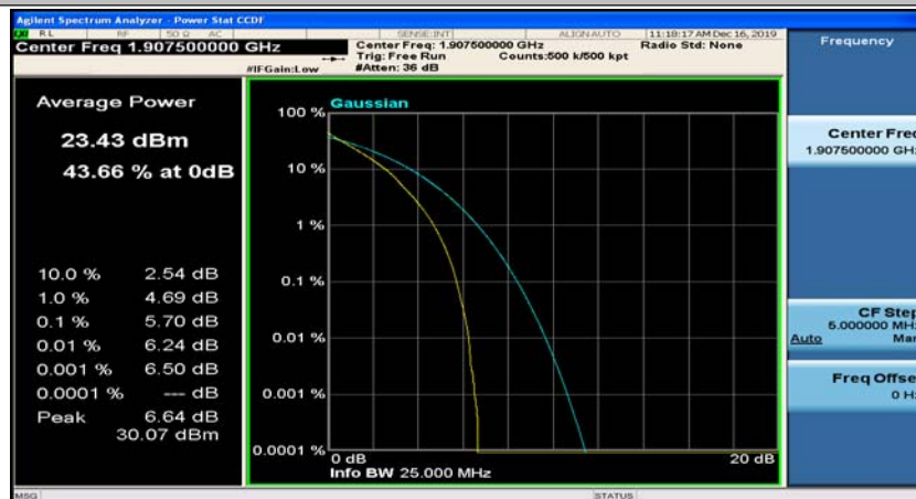
(Channel Bandwidth: 5 MHz)_HCH_QPSK_12RB#6
