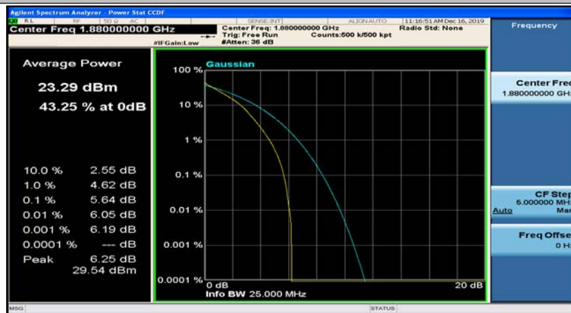
(Channel Bandwidth: 5 MHz)_MCH_QPSK_12RB#6
