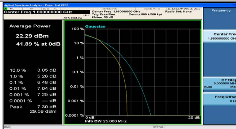
(Channel Bandwidth: 3 MHz)_MCH_16QAM_8RB#4
