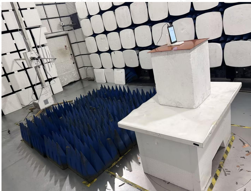
Radiated Emissions Measurement (Below 1GHz)
