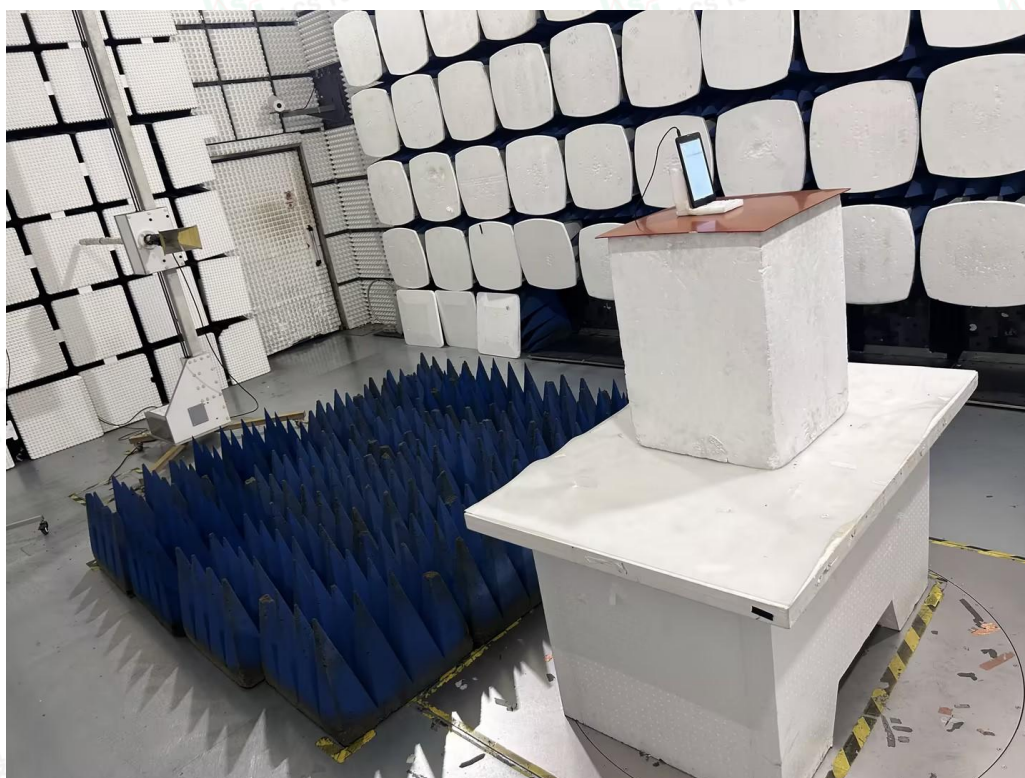
Radiated Emissions Measurement (Above 1GHz)
