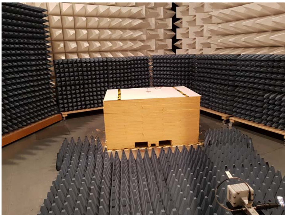
Figure 6 EUT / set up - test module ER3 (radiated emissions 18 - 30 GHz)
