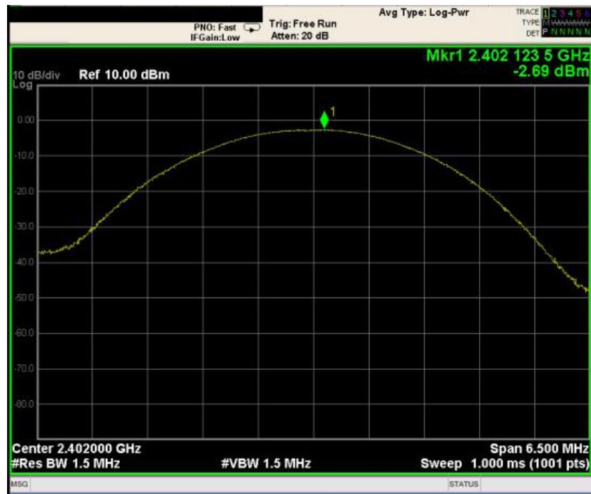
Peak output Power plot on channel 39 (2Mbps)
