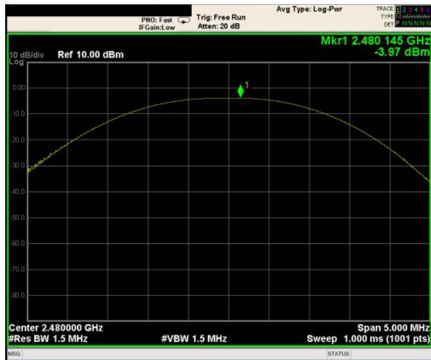
Peak output Power plot on channel 00 (2Mbps)
