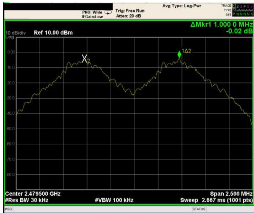
(1Mbps) Channel Separation plot on channel 77-78
