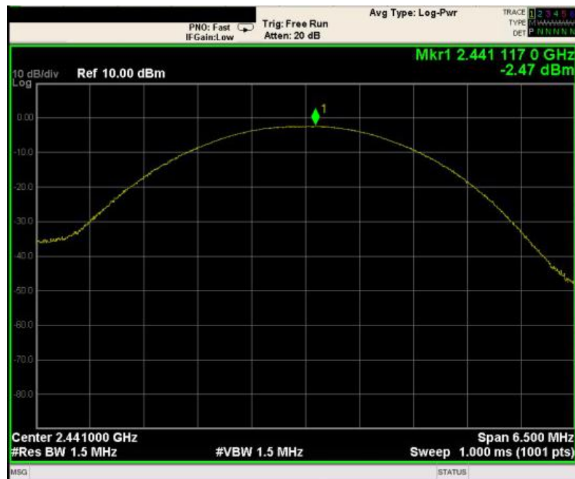
Peak output Power plot on channel 78 (2Mbps)
