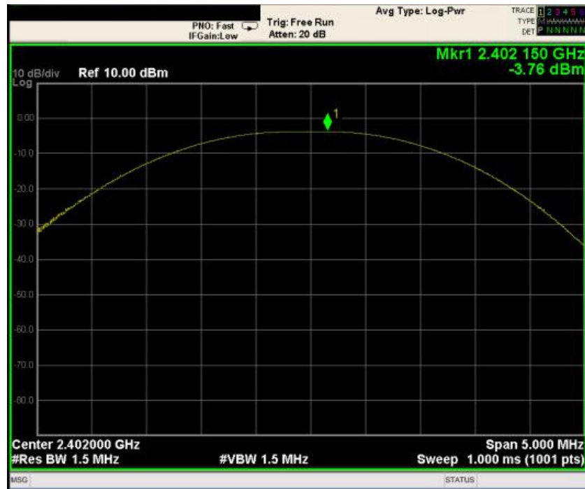
Peak output Power plot on channel 39 (1Mbps)
