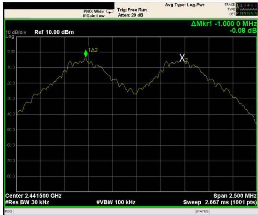
(1Mbps) Channel Separation plot on channel 39-40
