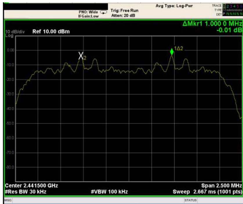
(2Mbps) Channel Separation plot on channel 39-40
