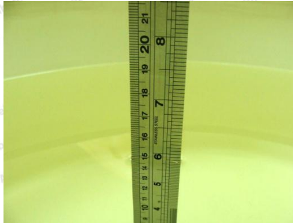
Photo of Liquid Height for Body SAR
