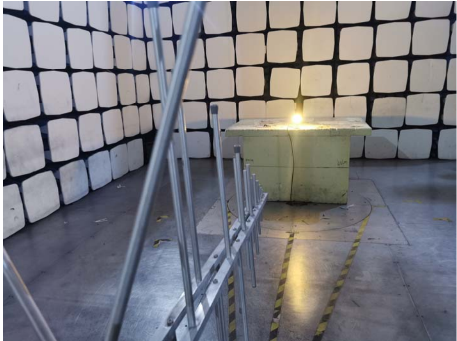
Radiation Emission Test Setup (30MHz to 1GHz)
