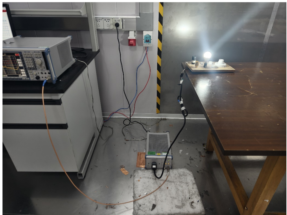
Conducted Emission Test Setup
