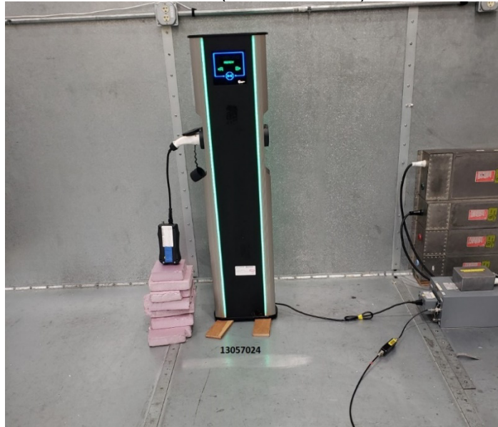
LINE CONDUCTED EMISSION (WITHOUT TAG)
