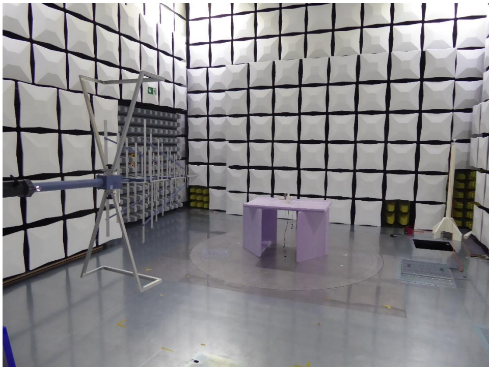
191836_02.JPG: Setup SAC E-field
