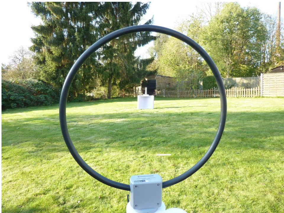
191836_04.JPG: Final measurement H-field outdoor
