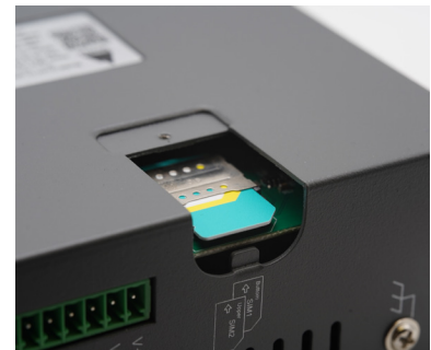
Figure 21. With one SIM fitted
