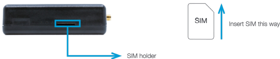
Figure 22. ZETA-NLP and ZETA-NSP - SIM holder
