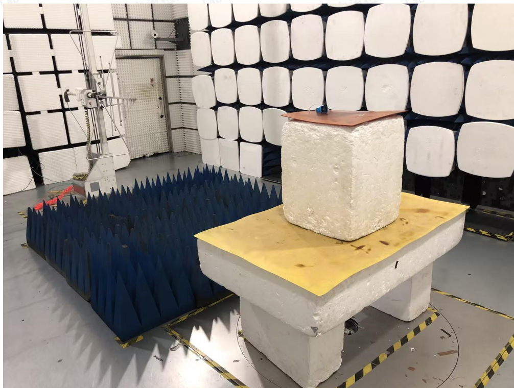
Radiated Emissions Measurement (Below 1GHz)
