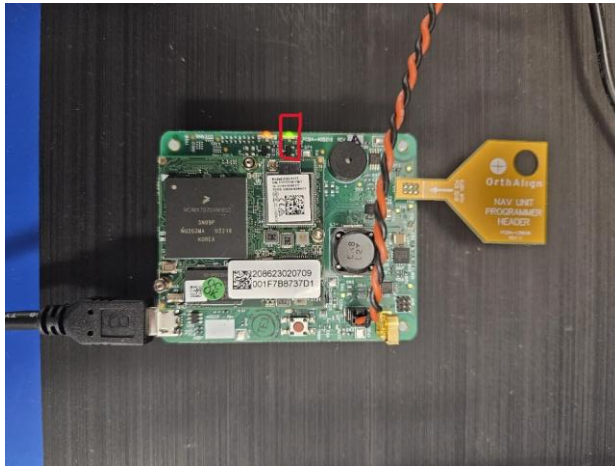
Figure 11- Green Light in a PCBA
