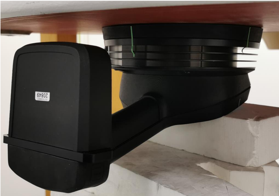
Figure 6 Front side of the DUT against the phantom, 0mm separation distance
