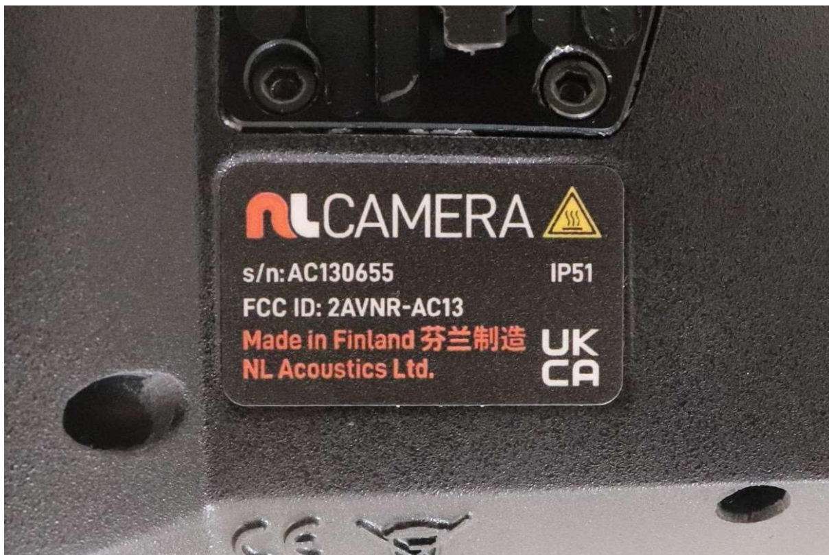
Photograph 3. The type label of the EUT
