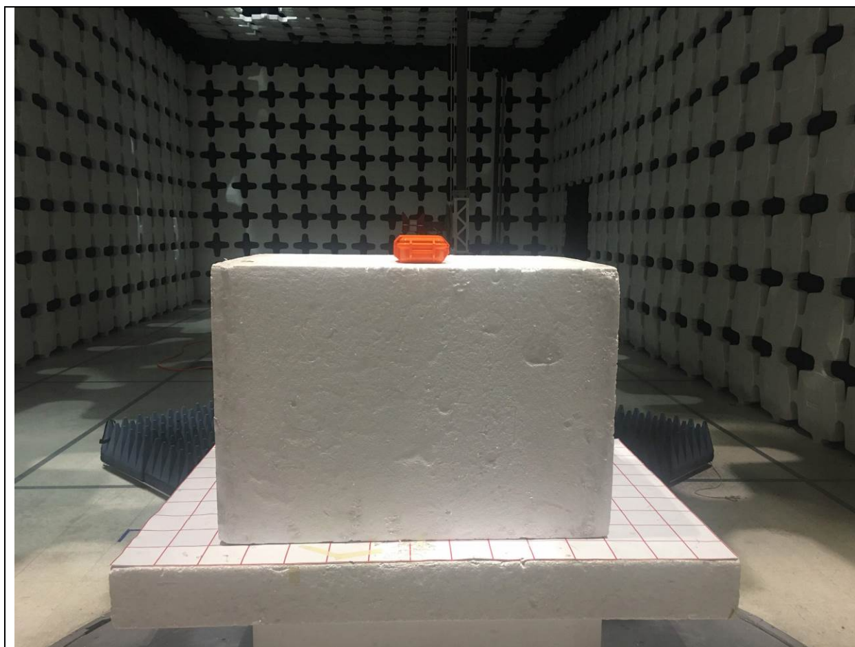
Radiated Emission Test above 1GHz Rear View
