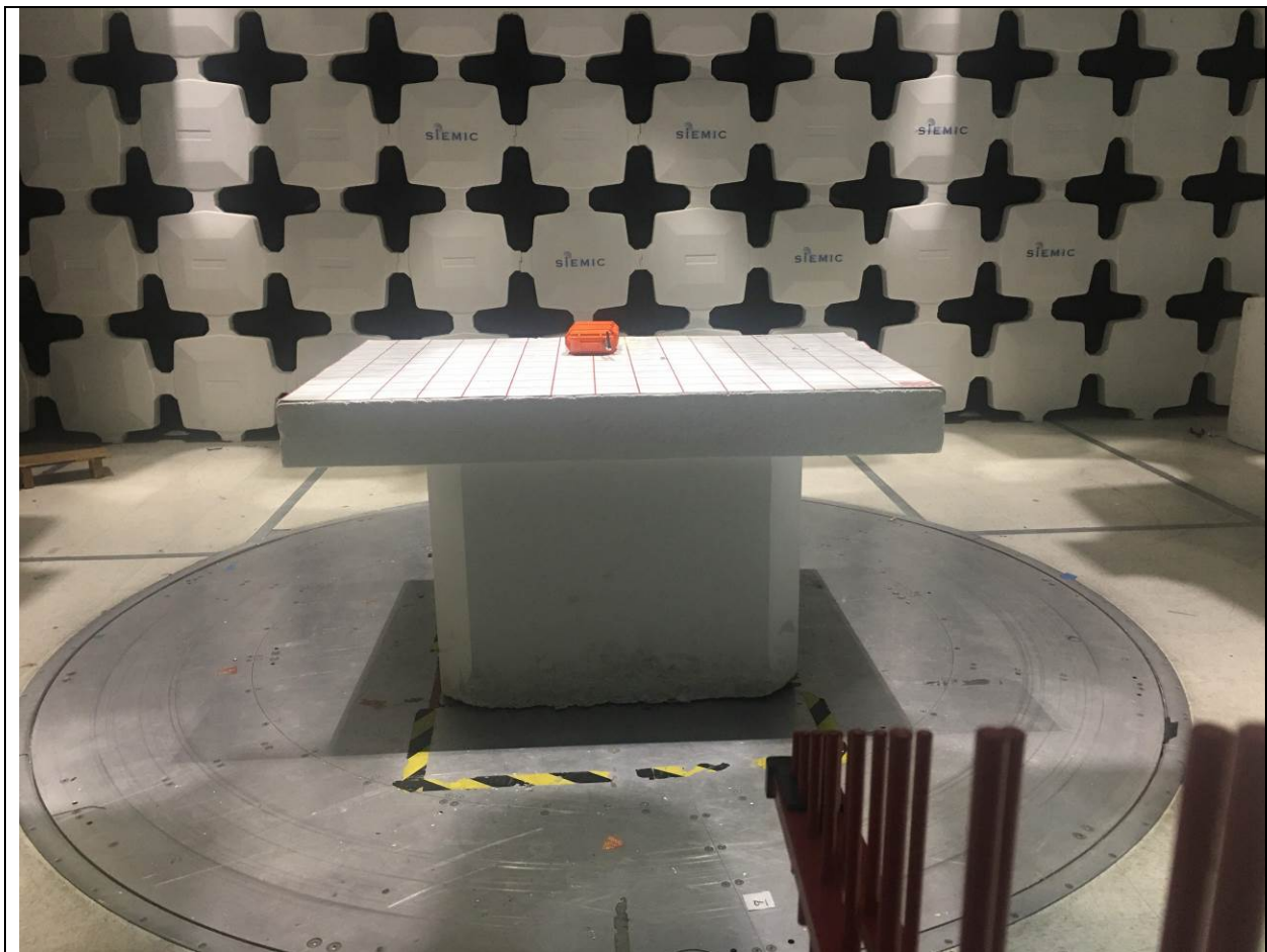
Radiated Emission Test below 1GHz Front View
