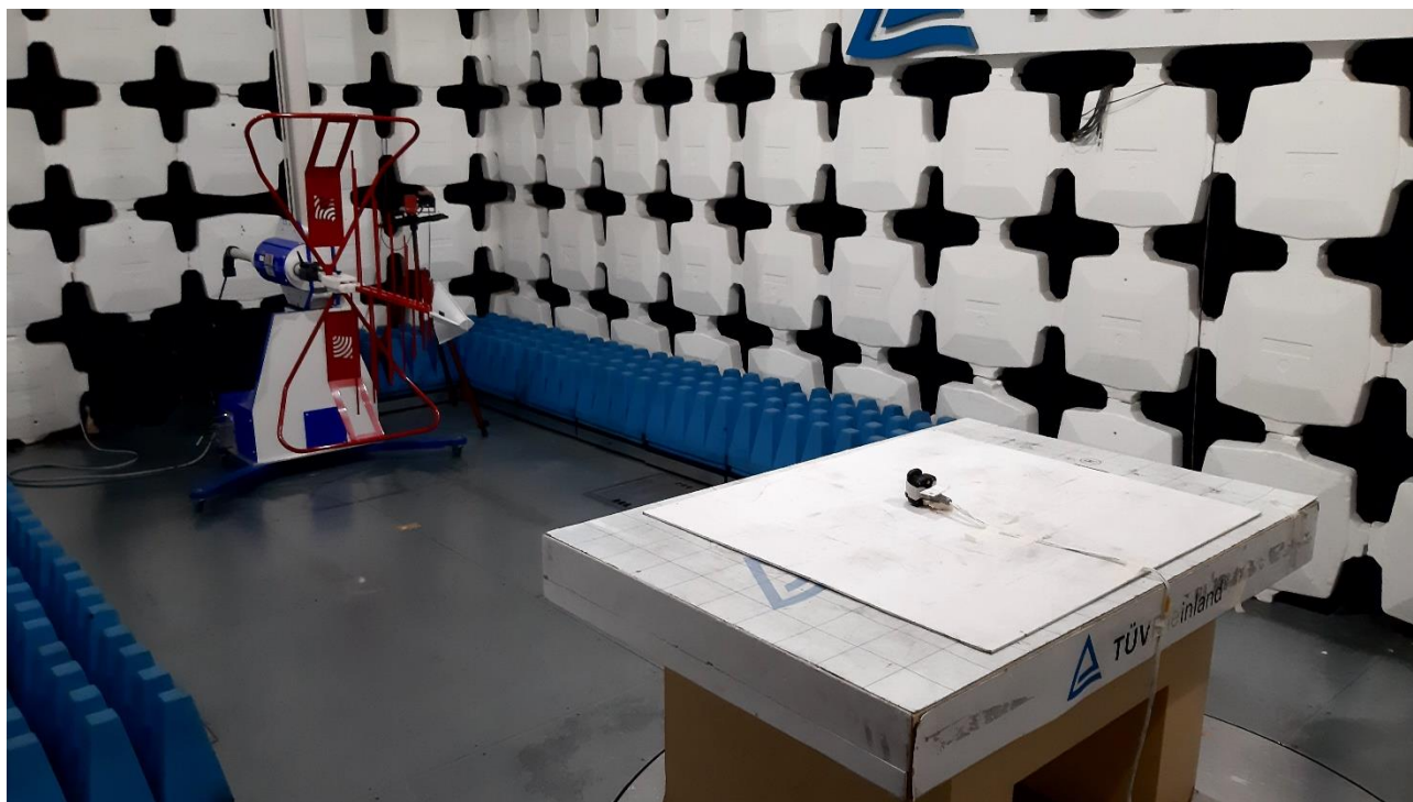
radiated emission test set-up (range 30-1000MHz)
