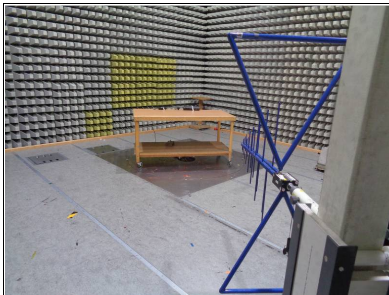
Figure 6-6: test setup for Radiated disturbances 30 MHz to 1000 MHz – Configuration mode 2
