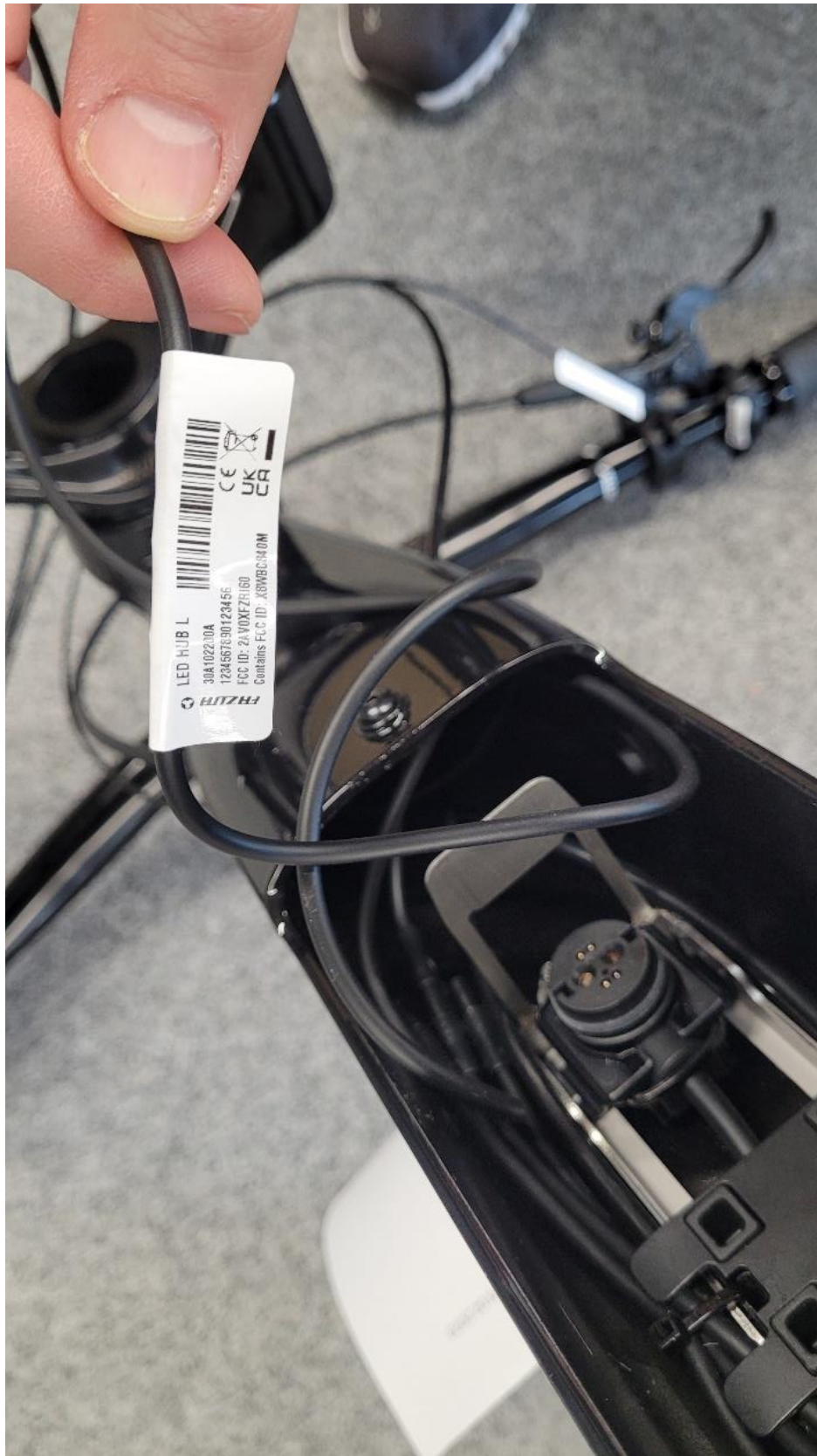
Figure 4-8: Display: LED HUB L, with product label incl. FCC information
