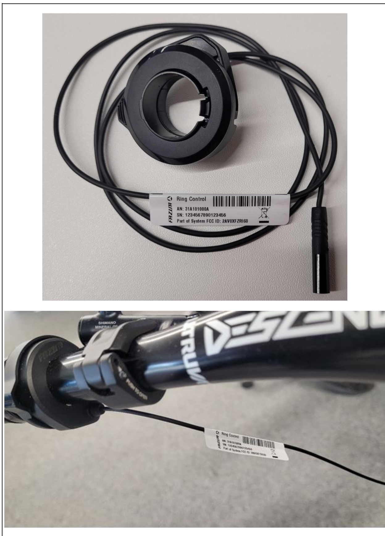
Figure 4-10: Remote: RING CONTROL, with product label incl. FCC information
