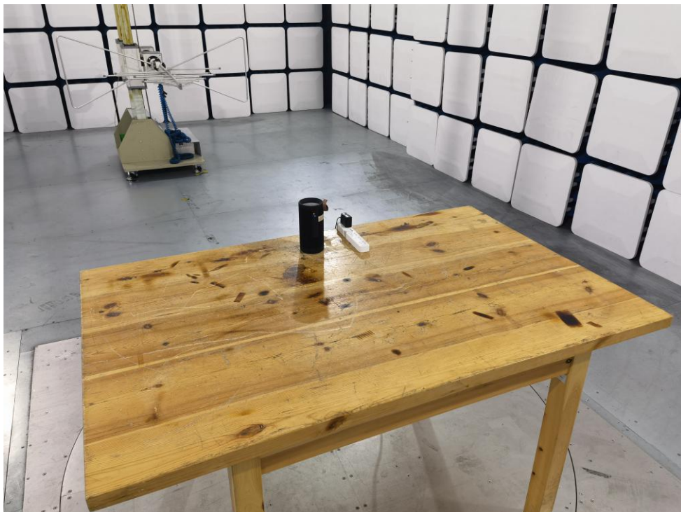
Photo of Radiation Emission Test
