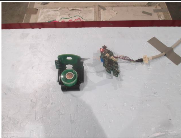
Figure 4: Test Setup Radiated Emission 9 kHz – 30 MHz – Configuration 1, 2, 3, 4
