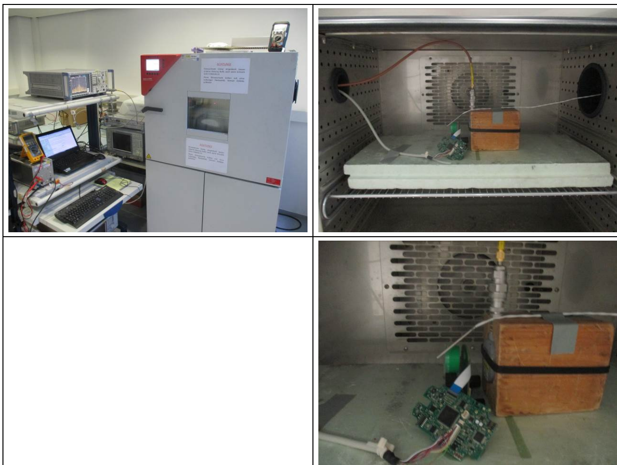
Figure 5: Test Setup – Frequency Stability with voltage or/and Temperature variation – Configuration 2
