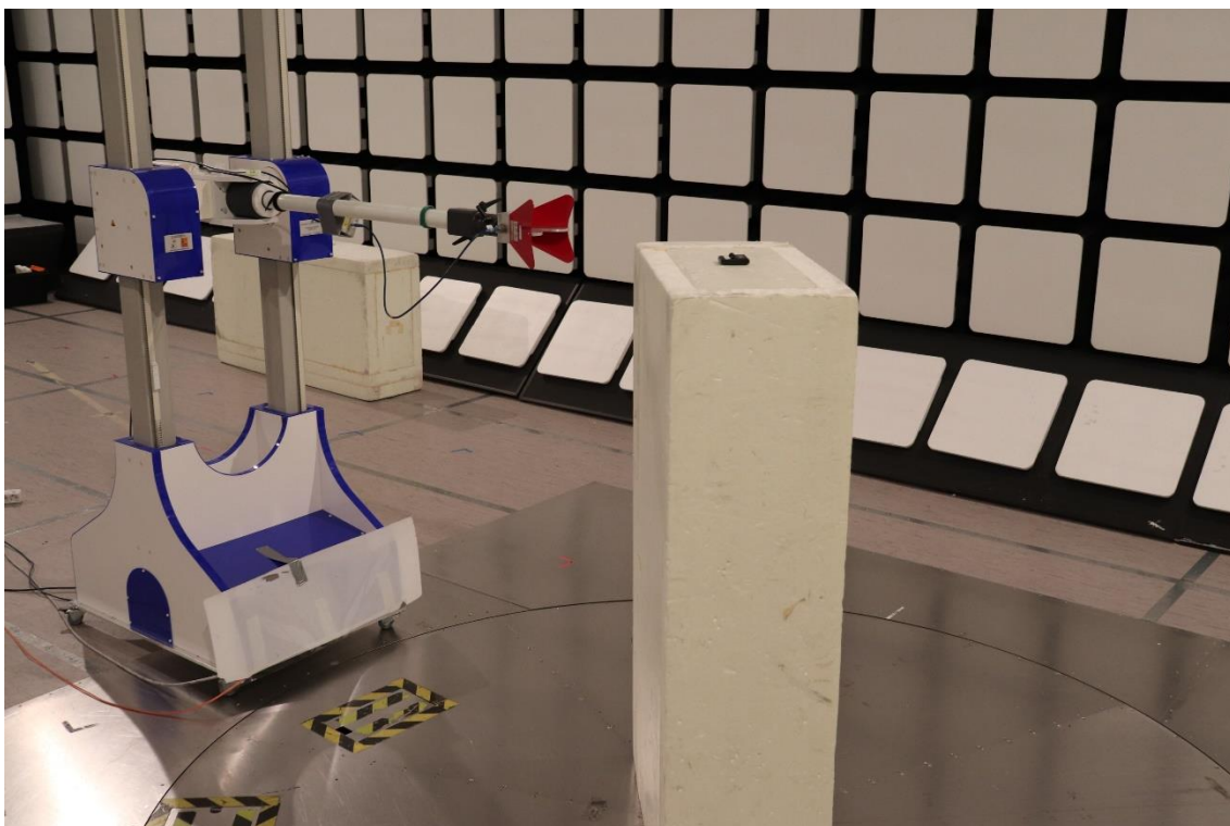
Photograph 8. Radiated Emissions 1 – 1.61 GHz and 10.6 – 18 GHz
