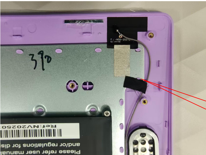
WiFi main antenna
