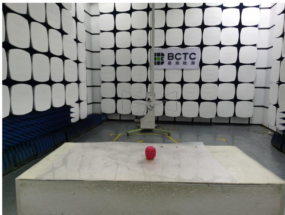
Radiated Measurement Photo (New IC+ Original Battery)
