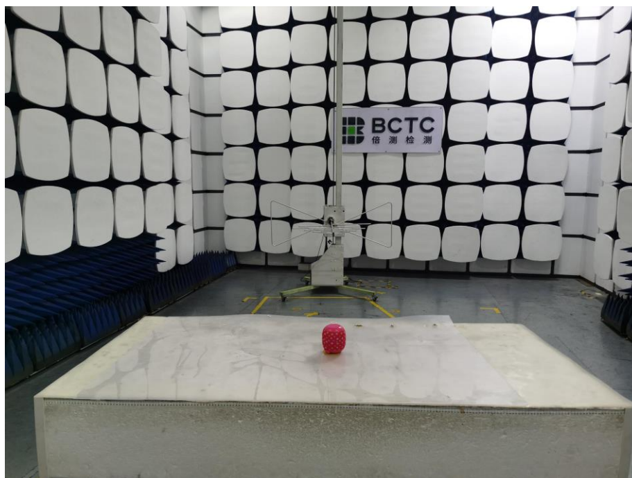
Radiated Measurement Photo (New IC+ New Battery)
