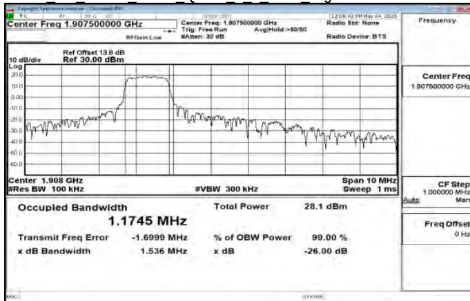
Cat M1 Band2 5MHz QPSK 6 0 Main HighCH19175-1907.5
