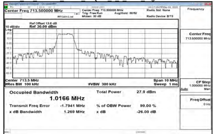
Cat M1 Band12 5MHz 16QAM 5 0 Main HighCH23155-713.5
