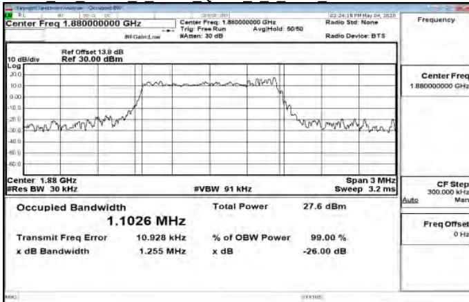
Cat M1 Band2 1 4MHz QPSK 6 0 Main HighCH19193-1909.3
