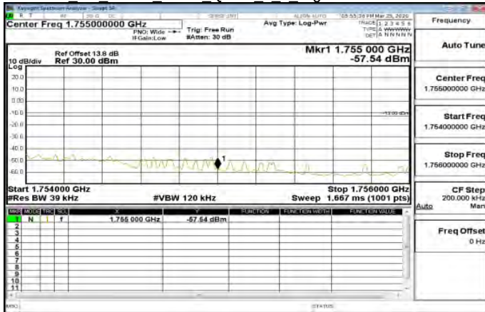
Cat M1 Band4 5MHz QPSK 1 0 LowCH19975-1712.5
