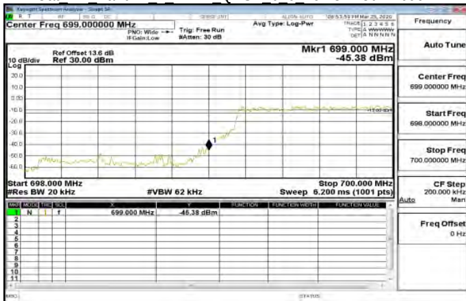
Cat M1 Band12 1 4MHz QPSK 6 0 LowCH23017-699.7
