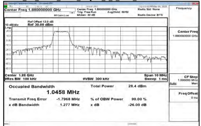
Cat M1 Band2 5MHz 16QAM 5 0 Main HighCH19175-1907.5
