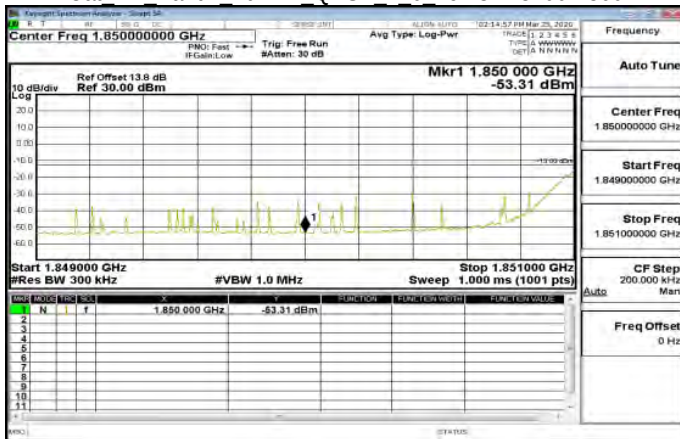
Cat M1 Band2 20MHz QPSK 1 0 LowCH18700-1860
