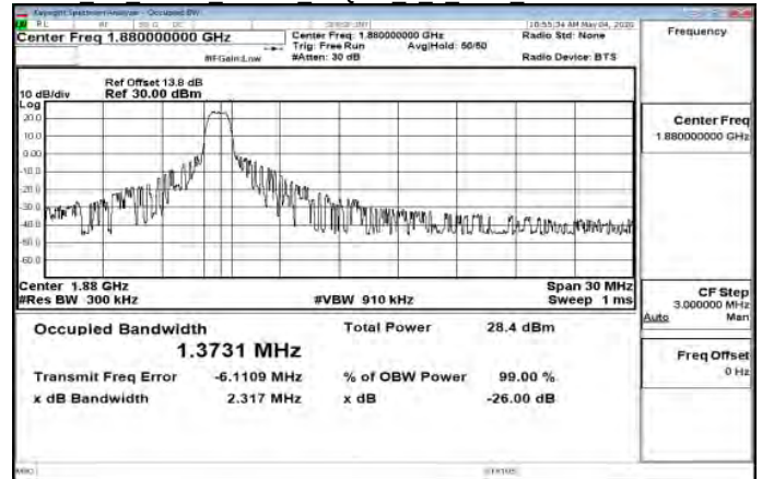
Cat M1 Band2 15MHz 16QAM 5 0 Main HighCH19125-1902.5
