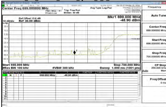
Cat M1 Band12 10MHz QPSK 6 0 HighCH23130-711
