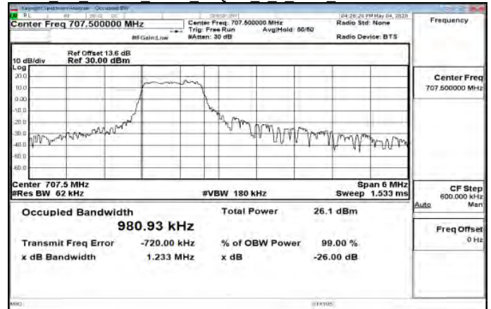
Cat M1 Band12 3MHz 16QAM 5 0 Main HighCH23165-714.5
