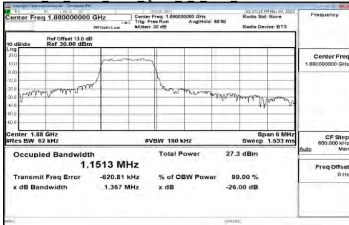
Cat M1 Band2 3MHz QPSK 6 0 Main HighCH19185-1908.5
