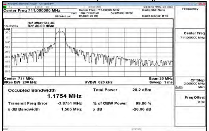
Cat M1 Band12 10MHz 16QAM 5 0 Main HighCH23130-711
