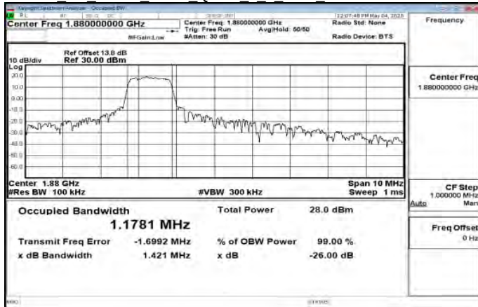
Cat M1 Band2 5MHz QPSK 6 0 Main HighCH19175-1907.5
