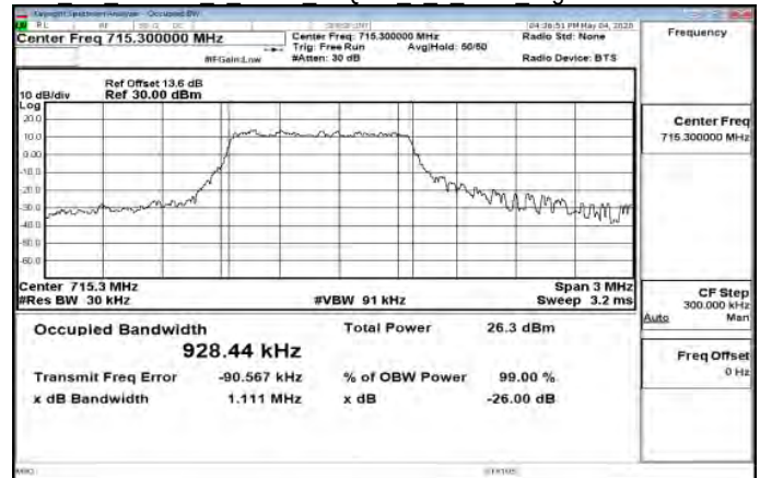
Cat M1 Band12 1 4MHz 16QAM 5 0 Main HighCH23173-715.3
