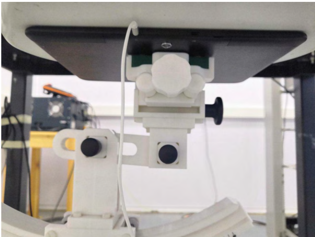
0mm body-worn Front Side Setup Photo (hotspot)
