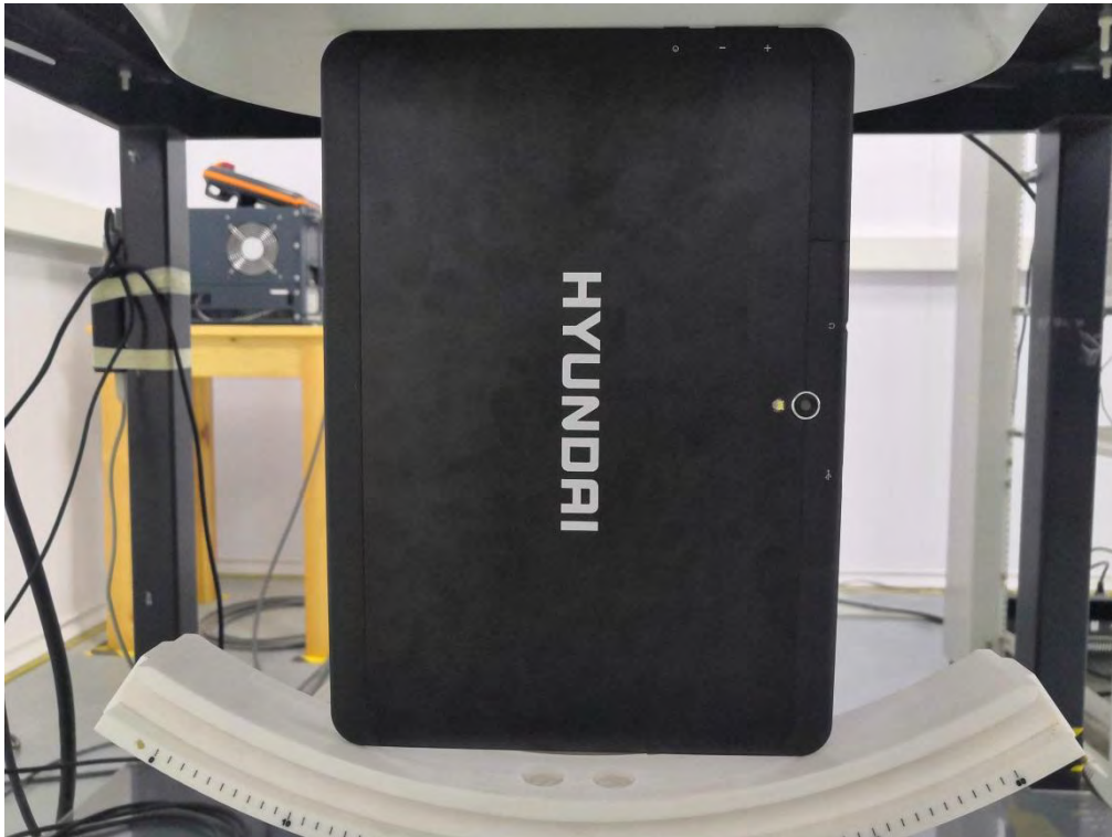
0mm body-worn Right Side Setup Photo (hotspot)
