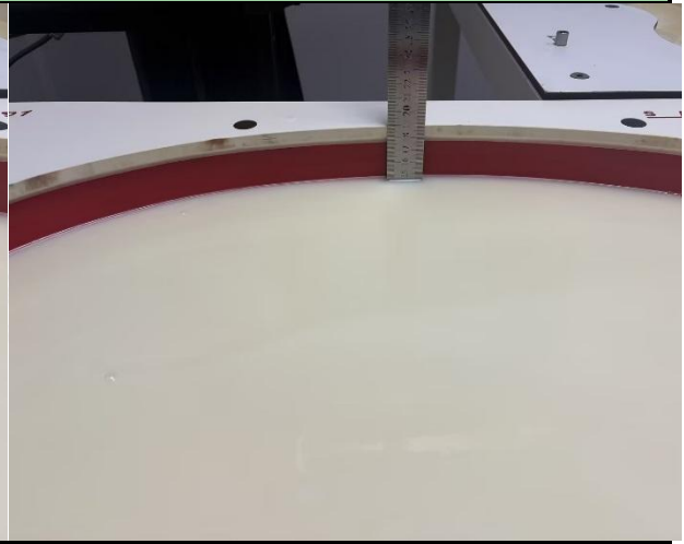
Photo 2: Tissue Simulant Liquid for Head 3000-8000
