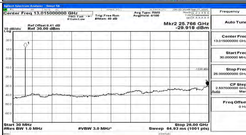
(Channel Bandwidth: 5 MHz)_LCH_QPSK_1RB#12
