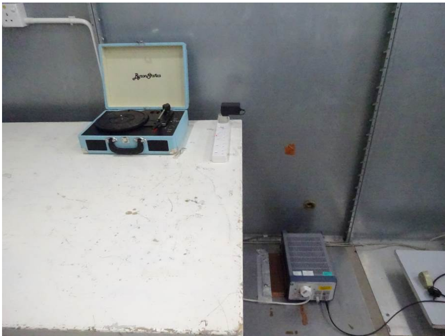
Measurement of Conducted Emission Test Set Up
