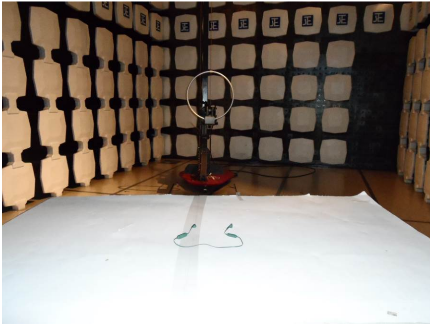
Measurement of Radiated Emission Test Set Up
