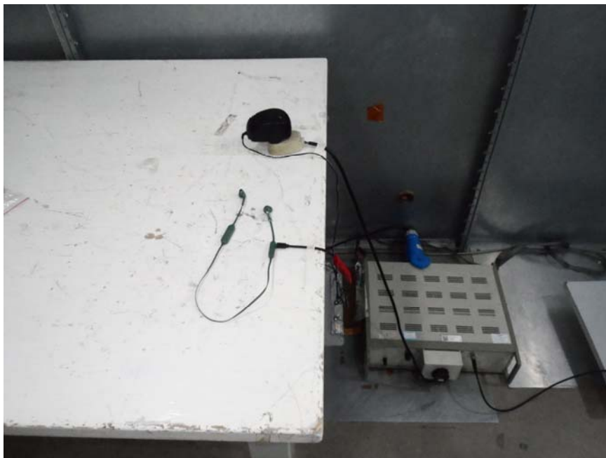
Measurement of Conducted Emission Test Set Up
