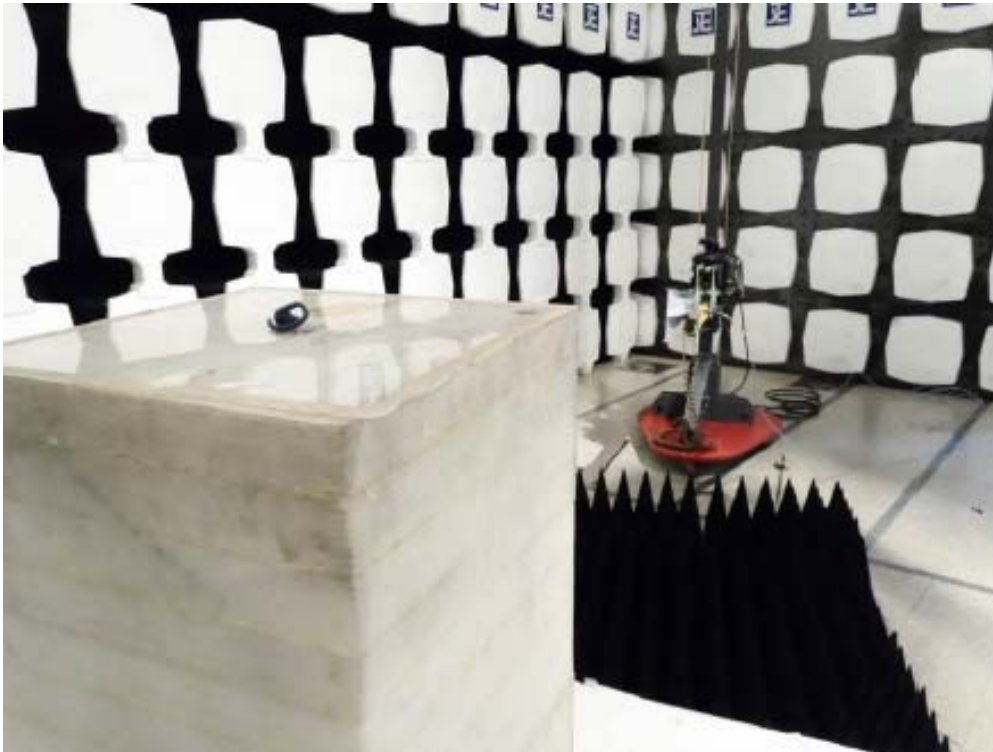
Measurement of Radiated Emission Test Set Up
