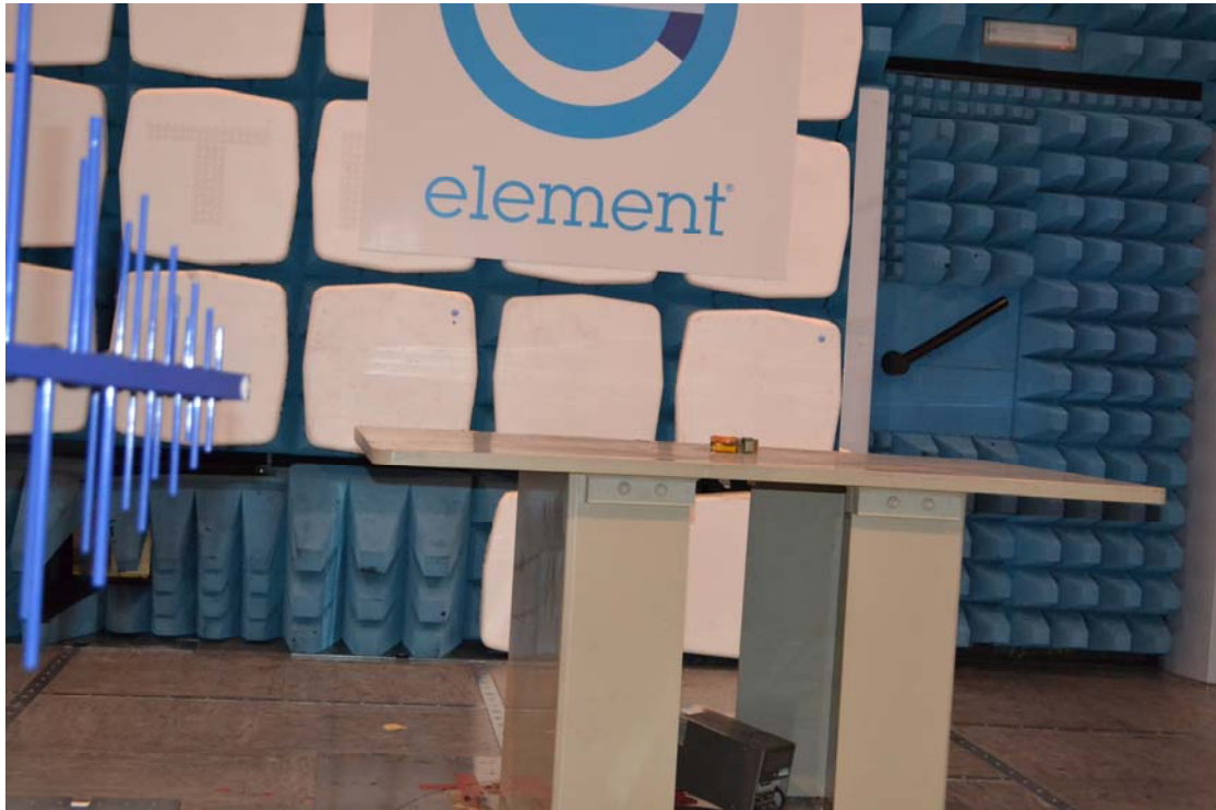
Radiated setup above 1 GHz
