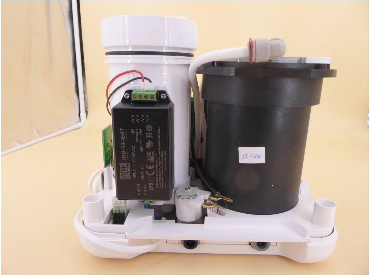
EUT, back side (AC/DC converter)
