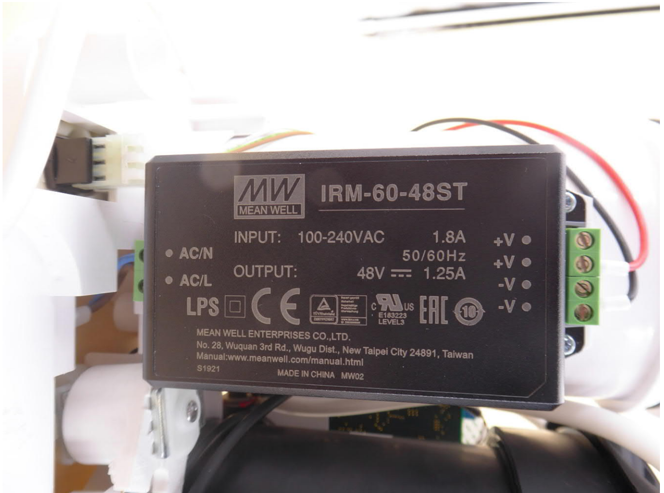
AC/DC converter, detail view
