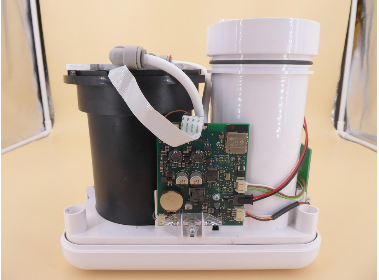
EUT, front side (main PCB)
