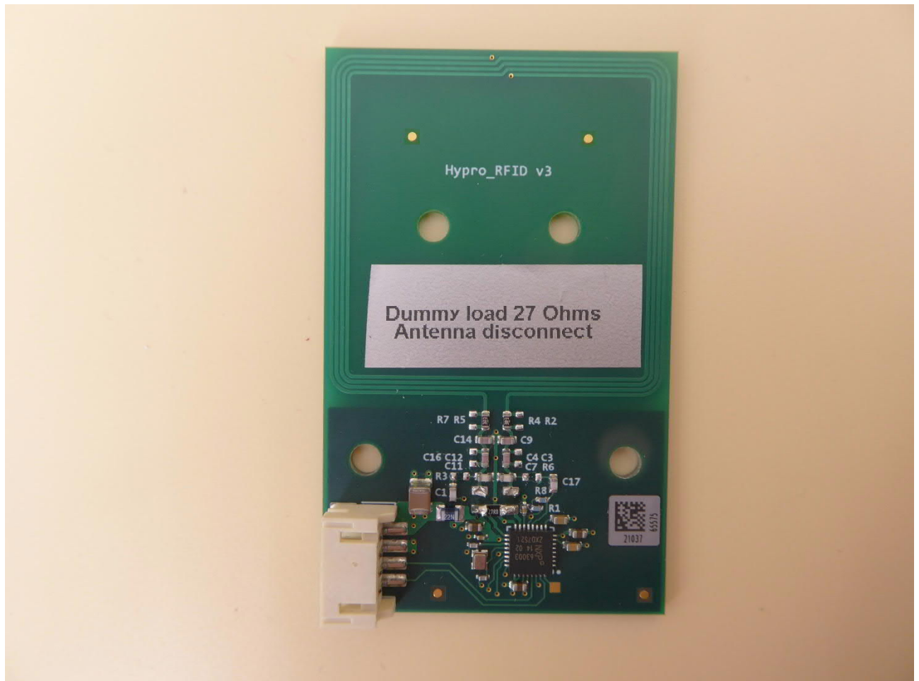
RFID PCB with dummy load, detail view
